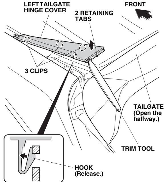
3. Remove the clip from the left tailgate hinge cover. Discard the clip, it will not be reused.
