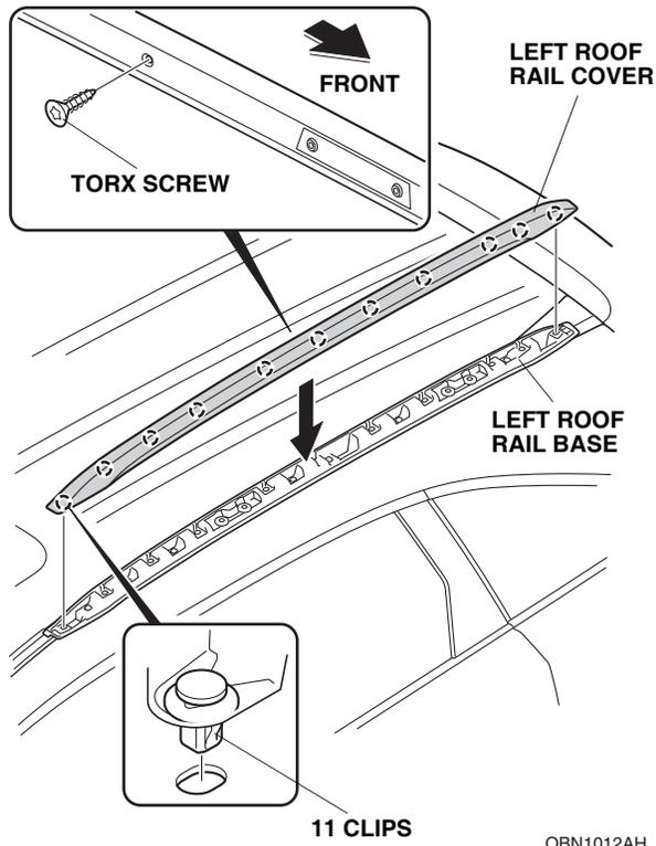
14. Secure the left roof rail cover to the left roof rail base with one TORX screw.
